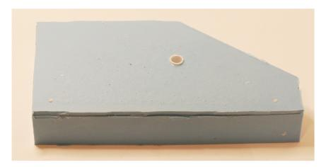
And a slow, careful pour of the resin was equally straightforward. I used the same TASK 4 resin that I had used for the front fenders and the resin was, once again, allowed to cure for 24 hrs.
