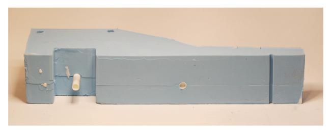
The lower mold was removed first, in a similar manner to removing the master from the molds.
