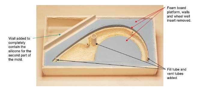
The exposed silicone surface was brushed with mold release (two coats) and, once it had dried thoroughly, the second part of the silicone mold was poured into the box and allowed to cure overnight.
