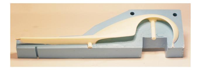
The upper mold covered the side wall of the running board so was more awkward to remove. Removing it after the lower mold was out of the way made most sense.
