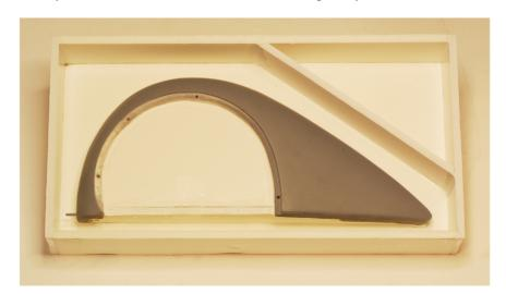
The mold box was then filled completely filled with silicone up to the top of the walls.
